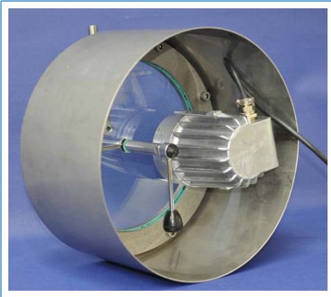
VETROLUX® sightglass similar to DIN 28120, DN 200, PN 0, with welded tube for wall mounting, centrally mounted wiper, spraying device and CHEMLUX® light fitting for hazardous areas, type FKEL 50 dH, 50 W, 24 V, Ex d IIC T3 Gb, Ex II 2 G + D
