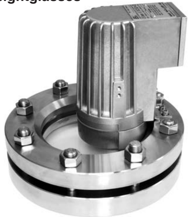
Type HEL 50 deHW, Ex d e o p is IIC T3 Gb, Ex t IIIC T195°C Db IP67, Ex II 2 G + D, 230 V, 50 W, halogen version, mounted on circular sightglass to DIN 28120, DN 125, PN 10, in 1 port version.
