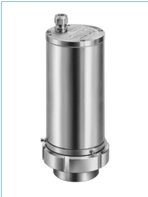
Sightglass light fitting type EdelEx G20 dHR 80 K1, 20 W, 230 V, Ex d IIC T5 Gb, Ex t IIIC T95°C Db IP67 Ex II 2 G + D, with intermediate flange collar fixation "R 80" mounted on a screwed sightglass similar to DIN 11851, PN 6, DN 80.
