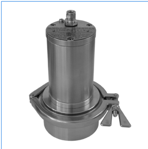
EdelLUX LED sightglass light fitting, type EdelEx LED, Ex d IIC T6 Gb, Ex t IIIC T80°C Db IP67, Ex II G + D, mounted onto metal fused sightglass for Triclamp® fittings, DN 50, PN 16
