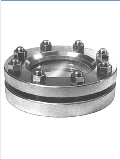
Complete assembly of sightglass fitting to DIN 28120, DN 100, PN 10, with glass disc of borosilicate to DIN 7080.
