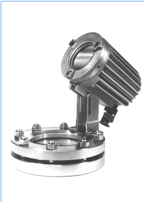
Complete assembly of sightglass fitting to DIN 28120, DN 125, PN 10, with glass disc of toughened sodium silicate to DIN 8902, fitted with CHEMLUX sightglass light fitting, type L 20 deH Sch, tilting hinge fixation
