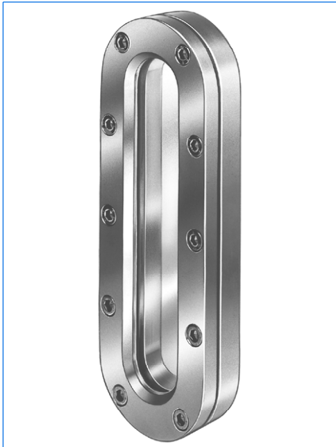
D-ended, elongated sightglass type LSGRR 316 Ti - 304-2,5-2-SL-8903-KLINGERSil-Silicone. Version with blind tappings, base and cover flange in stainless steel, PN 2,5, glass plate to DIN 8903, seals KLINGERSil C4400 / silicone, dimensions 341 x 116 mm.
