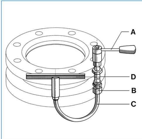
Assembly drawing of the wiper system WS
