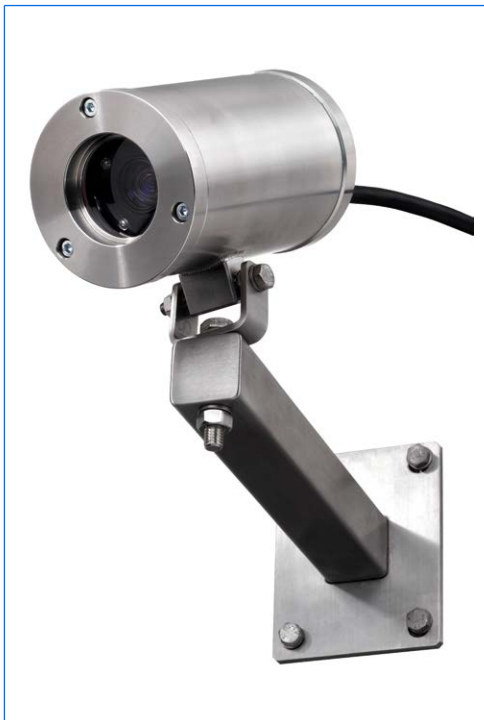
Ex camera Vario, stainless steel enclosure, Ex d IIB T6, Ex tD A21 IP67 T80°C, Ex II 2 G + D, with wall fixing system.
