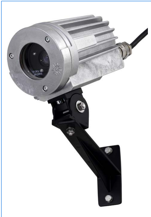
Ex camera Vario, aluminium alloy enclosure, Ex d IIC T6, Ex tD A21 IP67 T80°C, Ex II 2 G + D, with wall fixing system.
