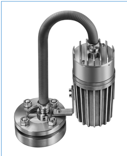
Fibre-optic lightpipe light fitting with built-in timer "U", type fibroLUX® 5035 W2 U sp, Ex de IIC T4 Gb, Ex t IIIC T130°C Db IP67, Ex II 2 G + D, 35W, 24 V AC, fixation of the light source by bracket "W", fixation of the lightpipe by universal support "W2" onto sightglass to DIN 28120, DN 40, PN 10
