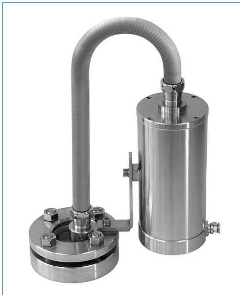
Stainless steel fibre-optic lightpipe light fitting, type fibroLUX E 5035 W2 sp, Ex d IIC T4 Gb, Ex t IIIC T130°C Db IP67, Ex II 2 G + D, 35 W, 24 V AC, fixation of the light source by bracket "W", fixation of the lightpipe by universal support "W2" onto sightglass to DIN 28120, DN 40, PN 10
