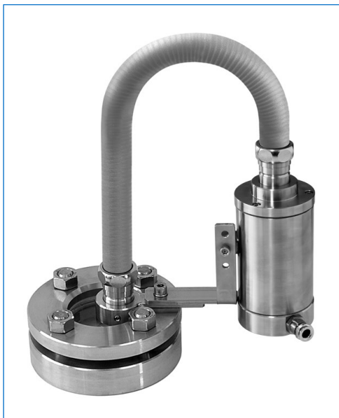
Stainless steel fibre-optic lightpipe light fitting, type fibroLUX E d PowerLED W W2 K2, Ex II 2 G + D, 7 W, 24 V AC / DC, fixation of the light source with bracket “W”, fixation of the lightpipe by universal support “W2” onto sightglass to DIN 28120, DN 40, PN 10
