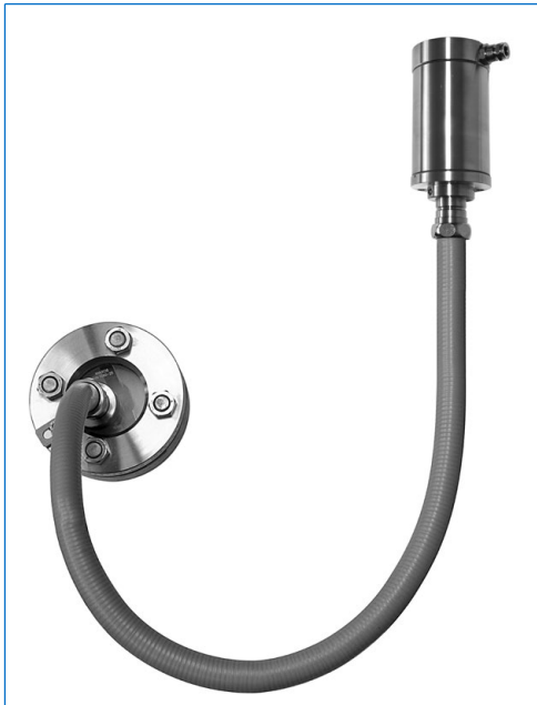
Stainless steel fibre-optic lightpipe light fitting for use in hazardous areas, type fibroLUX E d PowerLED Sch W2 K2, Ex II 2 G + D, 7 W, 230–240 V AC, fixation of the light source with tilting hinge “Sch”, fixation of the lightpipe by universal support “W2” onto sightglass to DIN 28120, DN 40, PN 10
