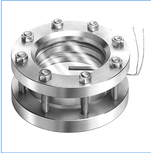
Double glazed sightglass similar to DIN 28120, DN 150, PN 16, with integrated heating element, 24 V, 50 W
