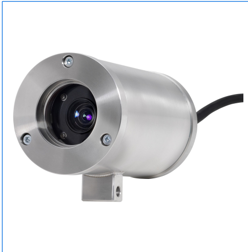
Ex camera niteZoom, stainless steel enclosure Ex d IIB T6, Ex tD A21 IP67 T80°C, Ex II 2 G + D.
