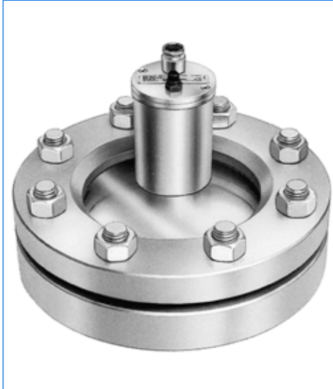
Sightglass light fitting type KVLR 20 HDW, 20 W, 24 V, with built-in momentary push-button "D", mounted with tilting hinge "Sch" on sightglass to DIN 28120, DN 100, PN 10, for application "view and light through one assembly".
